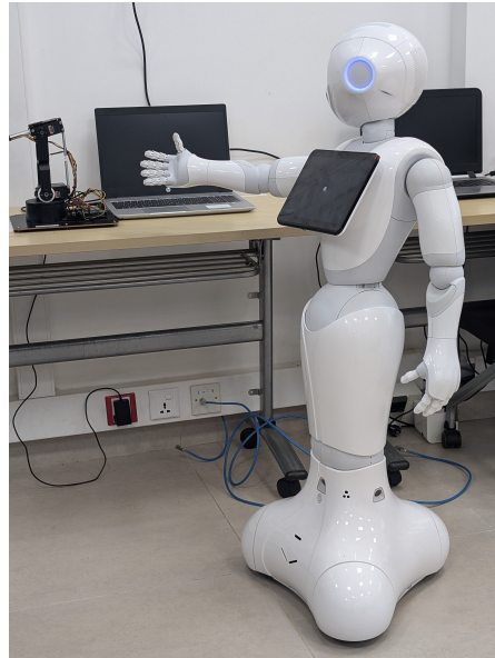
Figure 1: The Pepper robot performing a deictic pointing gesture during the experiment. Note that the robot's gaze is directed to the object to which it is gesturing. The picture is taken from the perspective of the user in the study.
