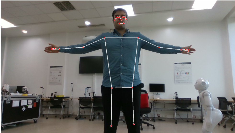
Figure 6: Skeletal model of the human demonstrator is estimated using Google’s MediaPipe pose estimation framework [5].
