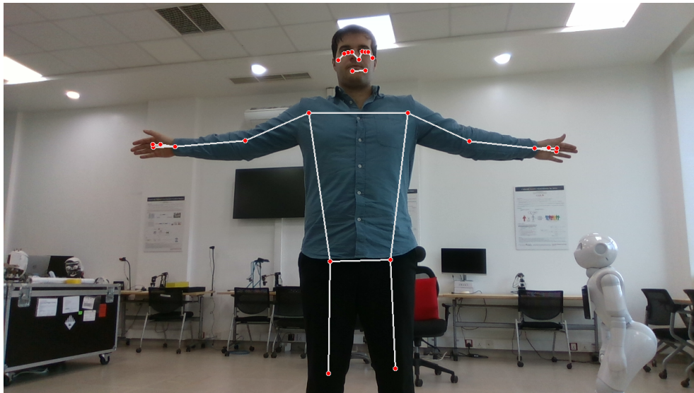
Figure 6: Skeletal model of the human demonstrator is estimated using Google’s MediaPipe pose estimation framework [? ].
